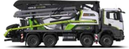
BEE MK28E PUMP MIXER Boom height: 27,15 m Boom sections: 4
